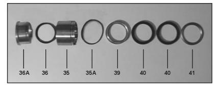
4. Remove the seal sleeve (35) from the manifold and/or crankcase. Remove the pressure rings (39&36A), v-sleeves (40&36), support ring (41) and o-rings (35A) from the manifold and seal sleeve, respectively. Examine seals carefully and replace if worn. Clean all parts.
